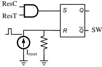
Fig. 5: Control logic for state switch.
