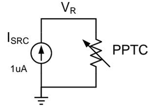
Fig. 7: Test circuitry for temperature domain.
